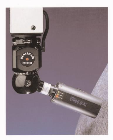
The OTP6M probe uses a visible laser beam which causes no distortion of component surfaces, allowing the inspection of pliable or delicate materials. The system gives repeatable Z-axis measurements and has an edge triggering capability. Typical applications include the measurement of interior parts for automobiles eg. seating and dashboards, plastic mouldings and clay models/prototypes.
